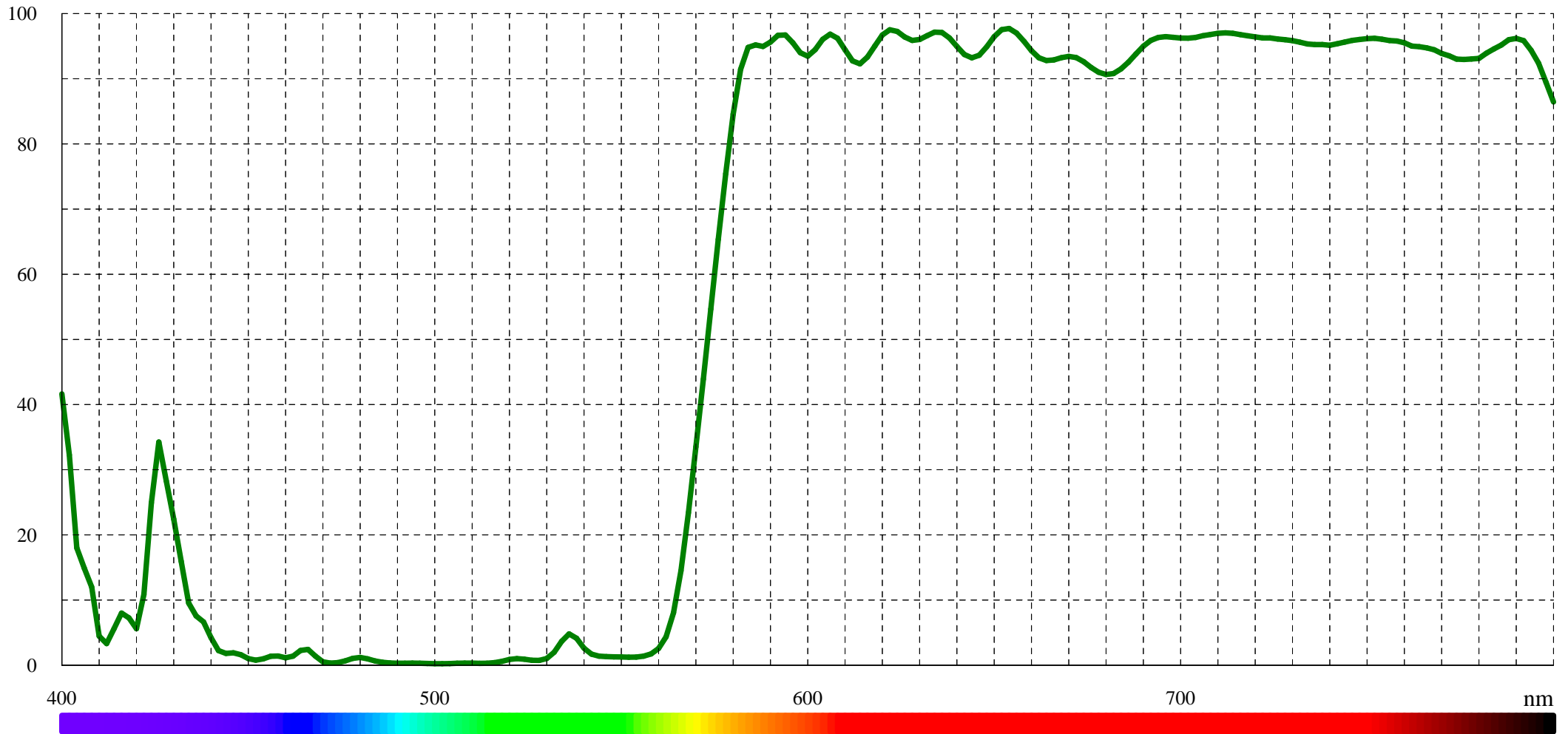
Typical transmission for DCLP 580 (LF101593)
