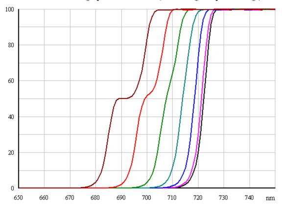
Tin % LWP720x3 Edge position vs AOI (0 - 30 Deg. Steps = 5 Deg.)
